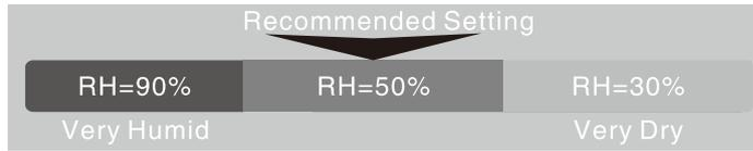
The TIMER MODE: This machine can automatically turn on/off depending on your humidity(%RH) setting. Timer mode is to allow you to switch the unit on/off at your desired time if you so desire.
